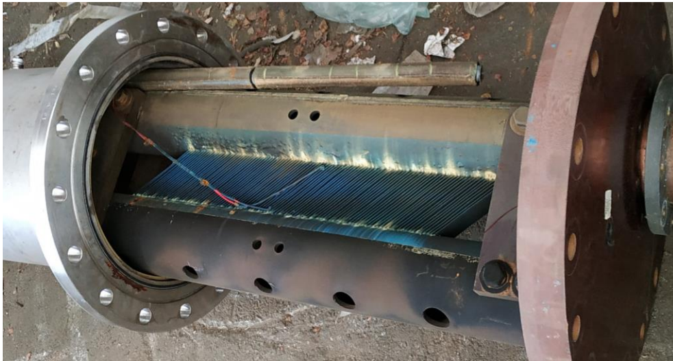
FIGURE 3: The current monitor shunt.
