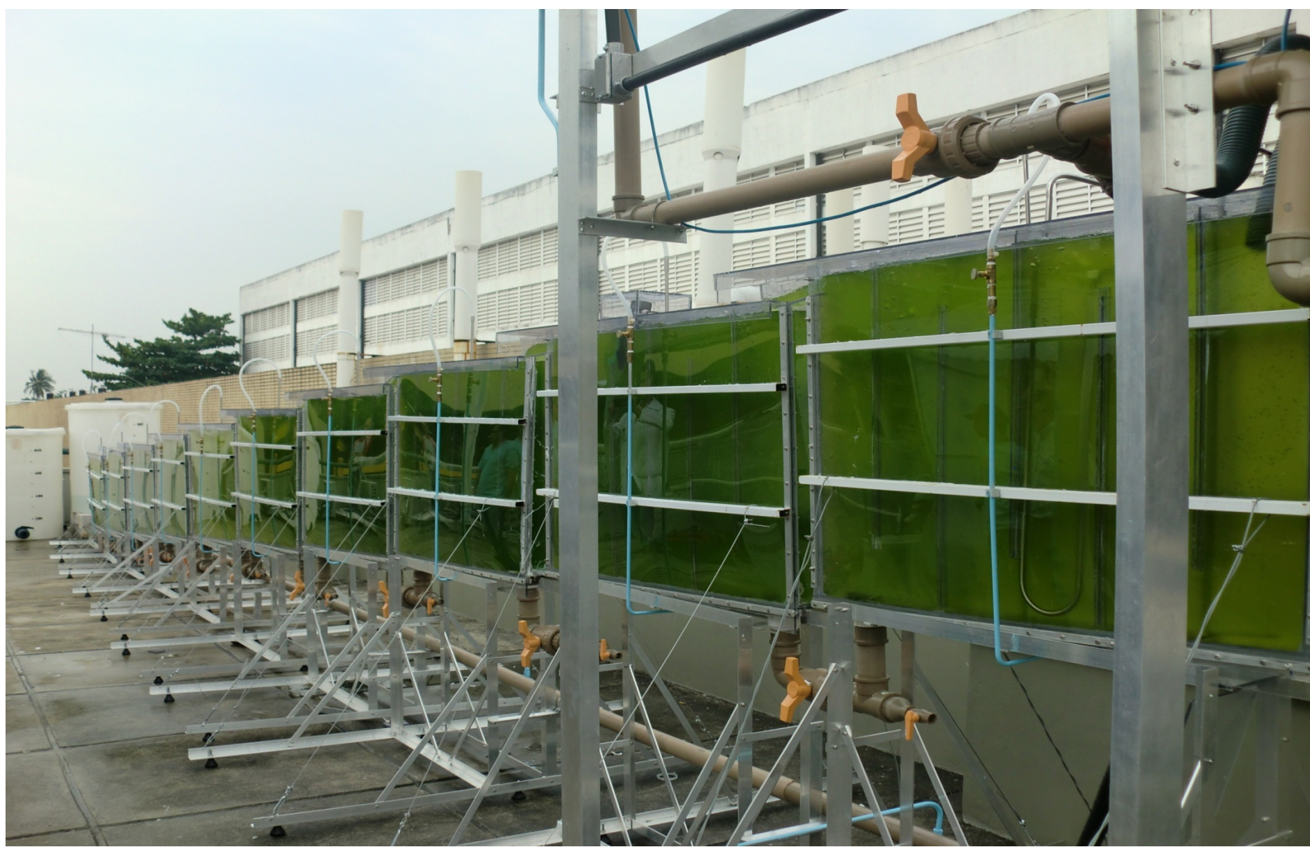
Microalgae produced in Photobioreactors (UFRJ) Lipids and Proteins: high production rates
