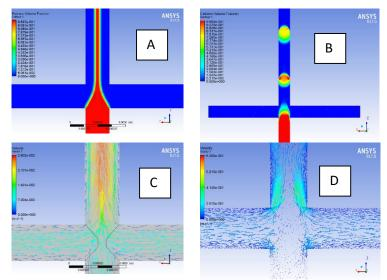
Figure 1 - a) Density profile for flow ratio 1: 1; b) Density profile for flow ratio 1:10; c) Velocity vectors for 1: 1 flow ratio; d) Velocity vectors for flow ratio 1:10.
