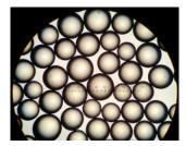
Figure 2 - Polymer particles obtained experimentally.
