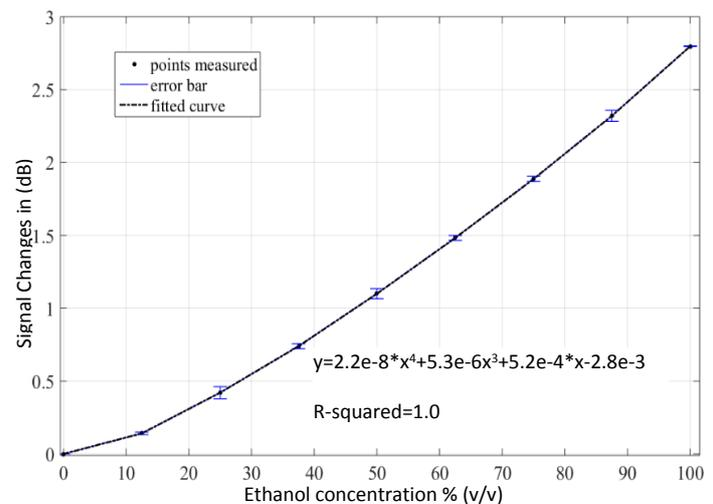
Fig.2 - SubTHz sensor response versus ethanol concentration.
