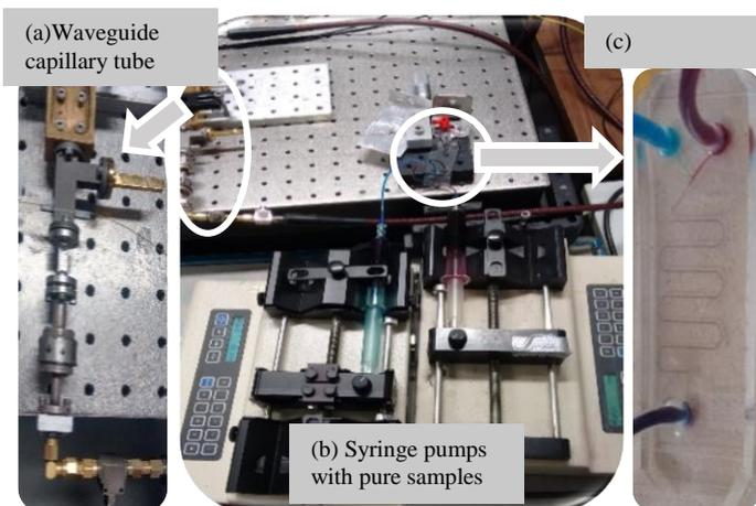
Fig.1 – Experimental setup. (a) Capillary tube integrated into a wave guide. (b) Syringe pumps and flow rate control. (c) Micromixer with blue dye color (ethanol), red dye color (in water) and purple as real liquid mixture along the microchannel.
