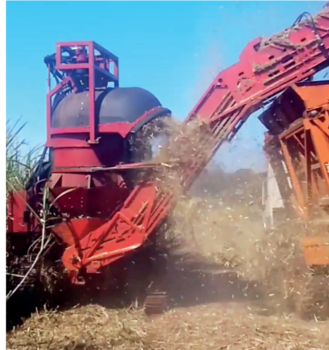
Assembly of the straw shredder/CTC in a commercial harvester from a mill partner, and operating in the field
