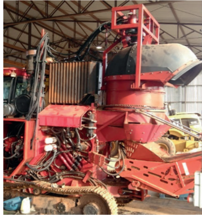
Assembly of the straw shredder/CTC in a commercial harvester from a mill partner, and operating in the field
