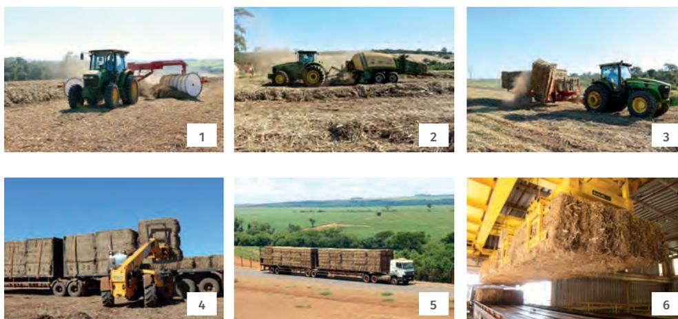
**Figure 17:** Overview of complete of Straw Baling system: straw windrowing, baling, collecting, loading and transporting bales, and bales processing plant.
