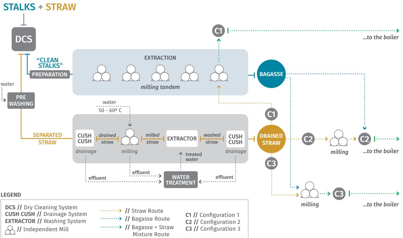
**Figure 61:** Process Flowchart: Configurations proposed by SUCRE for straw processing, C1, C2 and C3: Alternative 1, 2 e 3, respectively | Design credit: Luiz Nascimento/Comunicação CNPEM.
