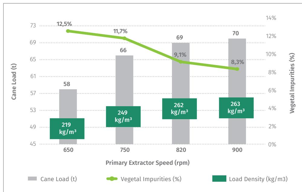
**Figure 21:** Field Trial – Cane Load versus Vegetal Impurities (wb) tested at four primary extractor speeds.
