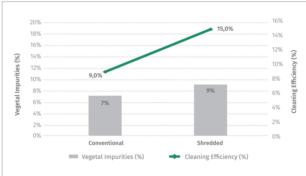
**Figure 26:** Efficiency of the DCS and percentages (%) of straw in the load in harvesting of approximately 50% of the straw available in the sugarcane field.
