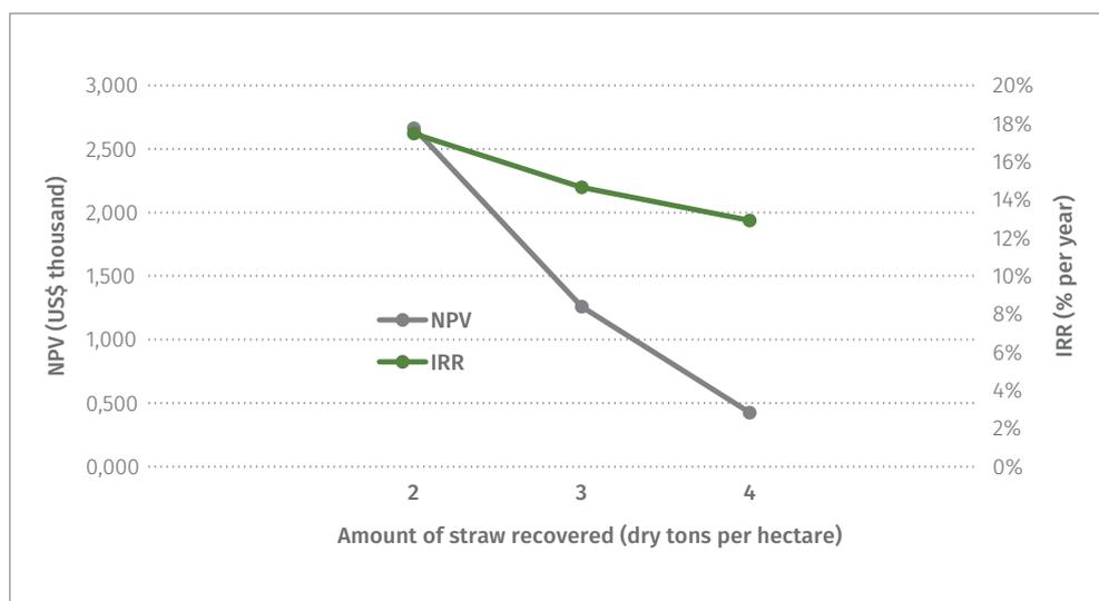
**Figure 70:** Sensitivity analysis of IRR and NPV to changes in the amount of straw recovered per hectare.
