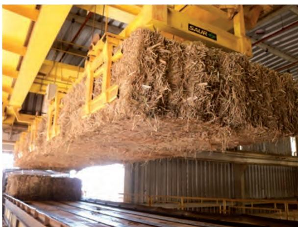
**Figure 40:** Automatic overhead crane for simultaneously unloading 10 bales (CTC).
