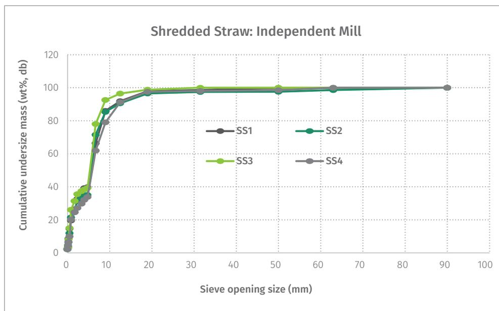
**Figure 59:** Cumulative undersize mass (wt%, db) as a function of the sieve opening size of shredded straw (independent mill) samples (SS1, SS2, SS3 and SS4) collected at Mill 7.
