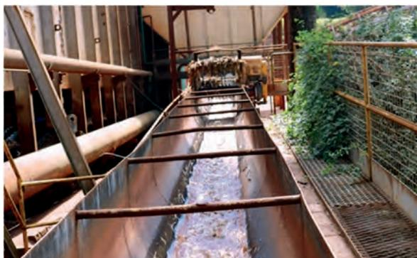
**Figure 53:** DCS separated straw washing and transporting in a water channel.
