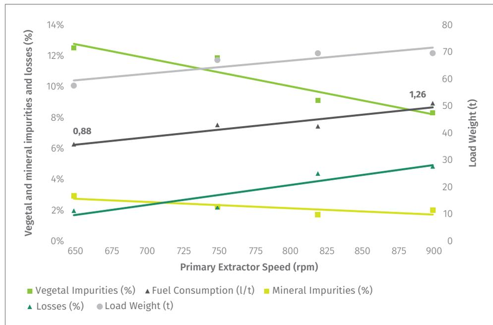
**Figure 22:** Effect of primary extractor RPM setting on each field variable.
