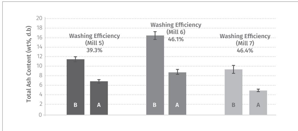
In addition, the washing process has been shown to promote the leaching of chemical elements that are critical for burning in boilers; these include silicon (Si), potassium (K), sulfur (S), and chlorine (Cl). Lastly, it was noted that leaching efficiencies can reach greater values in optimized washing processes.
