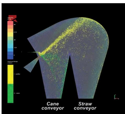
**Figure 31:** Standard model DCS in coupling CFD and Discrete Element Method (DEM).
