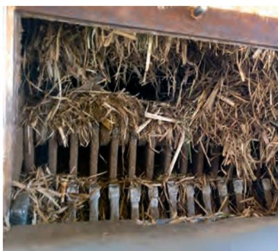
**Figure 42:** View of the hammer shredder.
