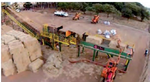
**Figure 39:** Unloading Straw Bales using adapted Cane Loader Machinery (Mill 2).
