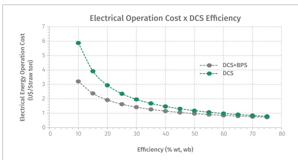
**Figure 52:** Electrical Energy Operating Cost in USD/ton (BRL/USD 3.25, 2018); DCS: Dry Cleaning System; BPS: Bale Processing System, Data: Considering Electrical Energy Price USD 50 /MWh.
