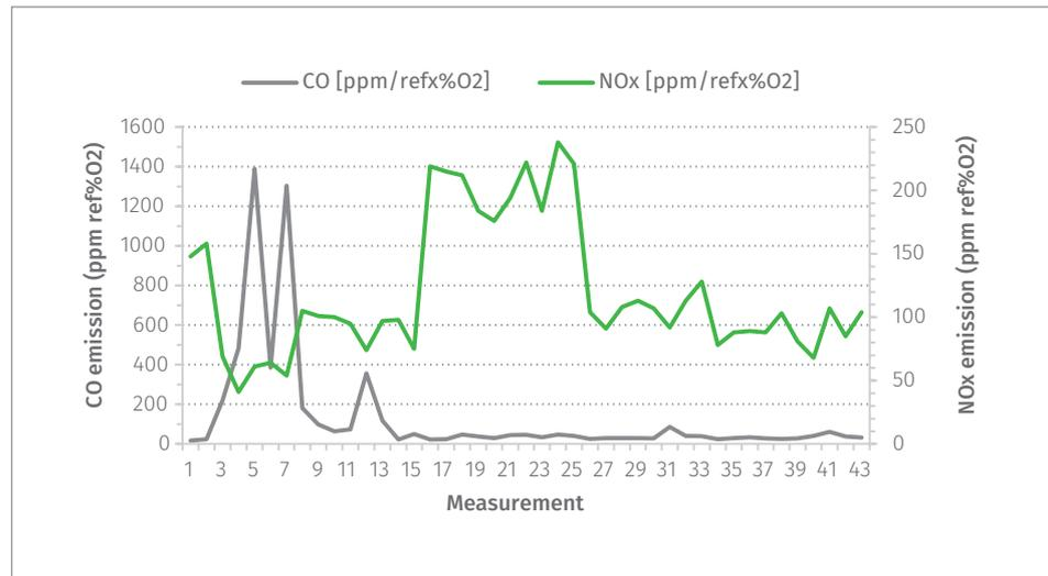
**Figure 64:** Relationship between CO and NOx emission in boiler.
