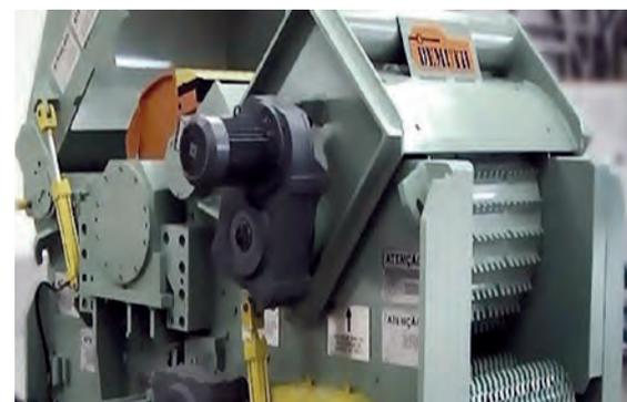
**Figure 41:** Rotary screen for straw cleaning.
