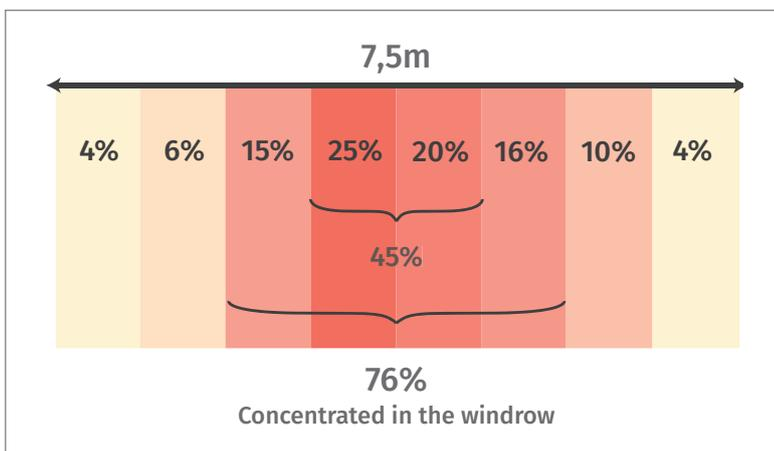
**Figure 18:** Distribution of residual straw after passing the baler.
