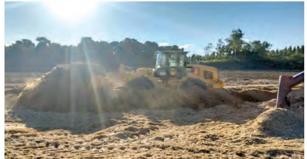
**Figure 47:** Bagasse and straw mixing by a tractor-type backhoe.
