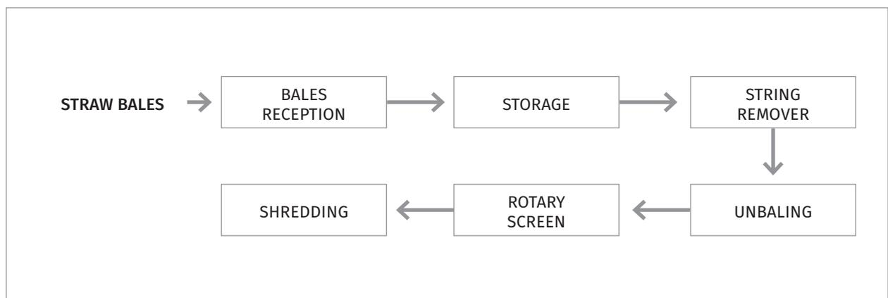
**Figure 38:** Unit Operation of Straw Bale Processing – Benchmark Case – Mill 3.
