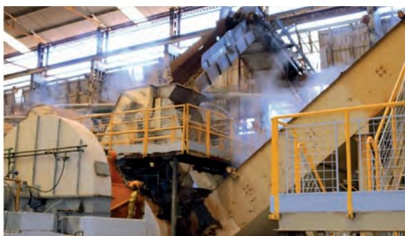
**Figure 55:** Straw feeding into the last mill of the milling tandem.
