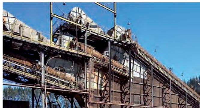
**Figure 50:** DCS with downward air blowing.
