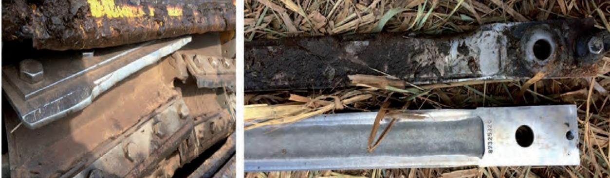
**Figure 49:** Wear of hay harvester knives and counter-knives.
