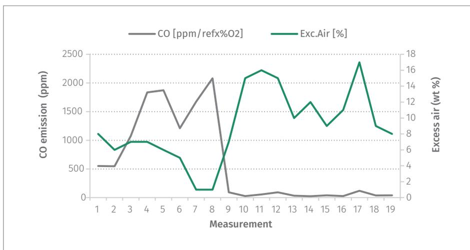
**Figure 63:** Relationship between CO emissions and excess air.
