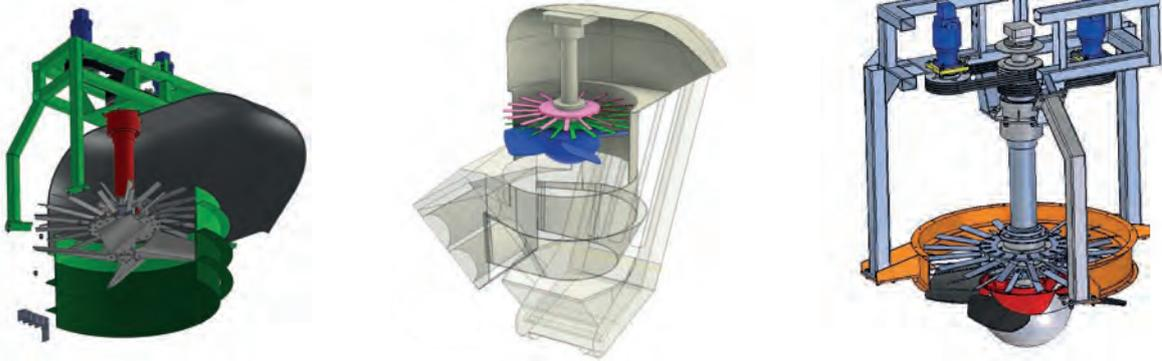
**Figure 23:** Straw Shredder, set of rotary knives (green) / counter-knives (pink), mounted on the primary extractor of the commercial chopped cane harvester.
