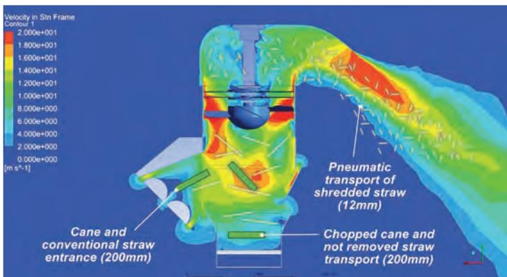
**Figure 29:** Straw Shredder in CFD (Computational Fluid Dynamics).
