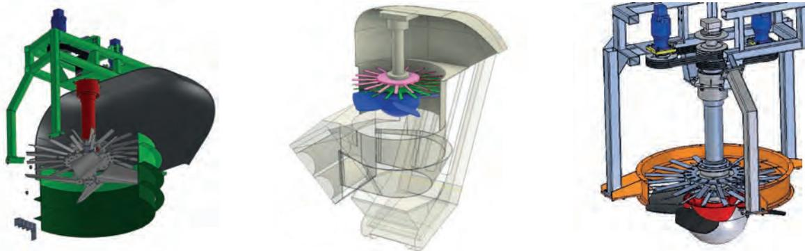
all cane straw material, which is blown by the primary extractor, through one set of rotary knives and counter-knives (RLT-053, 2018; RLT-069/01, 2019; Neves et al., 2015; Neves et al., 2016)<sup>7</sup>.
