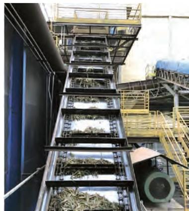
**Figure 54:** Washed straw drainage in the cush-cush screen.
