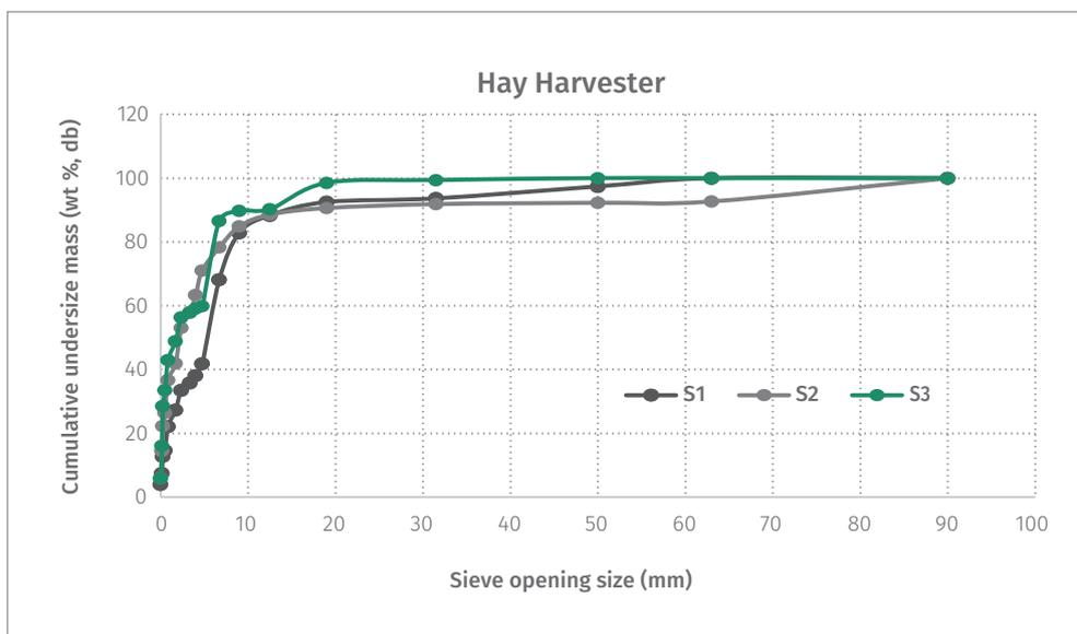
**Figure 48:** Cumulative undersize mass (wt %) as a function of the sieve opening size of bulk straw (hay harvester) samples (S1, S2 and S3).
