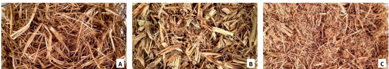
**Figure 60:** Typical appearance of straw processed by conventional hammer shredder (A), straw shredded in an independent mill (B) and bagasse-straw mixture produced through the straw feeding in the last mill of the milling tandem (C).
