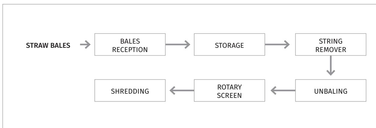
**Figure 38:** Unit Operation of Straw Bale Processing – Benchmark Case – Mill 3.
