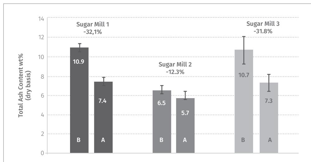
**Figure 45:** Ash content reduction before (B) and after (A) straw processing.
