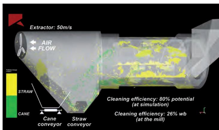
**Figure 32:** Virtual prototyping: alternative DCS during the CFD + DEM analysis (Scenario 1).
