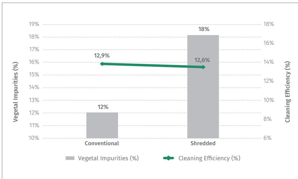
**Figure 27:** Efficiency of the DCS and percentages (%) of straw in the cane load in the harvesting of 100% of the straw available in the sugarcane field.
