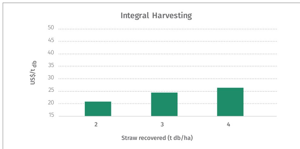
**Figure 34:** Straw recovery cost for different straw quantities, on dry basis, per hectare.
