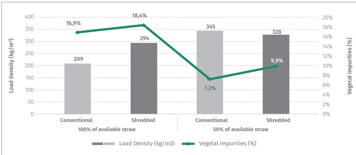
**Figure 28:** Load densities and vegetal impurities for shredded and conventional straw.
