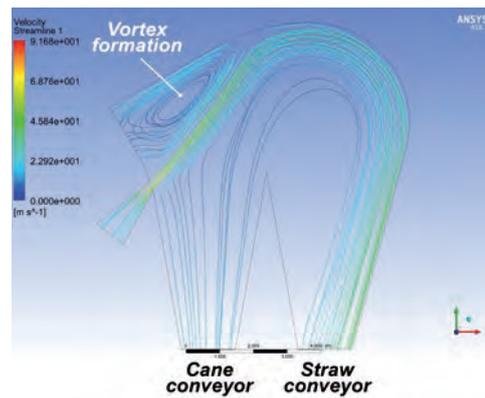
**Figure 30:** Standard model DCS in CFD (Computational Fluid Dynamics) indicating vortex formation.
