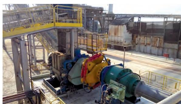
**Figure 56:** Independent mill for straw shredding.
