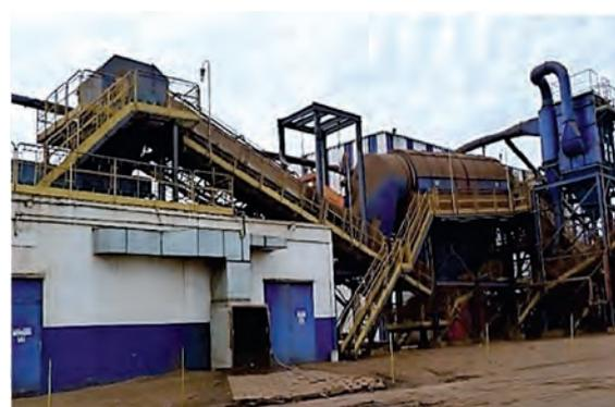
**Figure 44:** Model Straw Bale processing with a dust collection system installed in mill M3.
