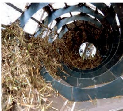
**Figure 41:** Rotary screen for straw cleaning.
