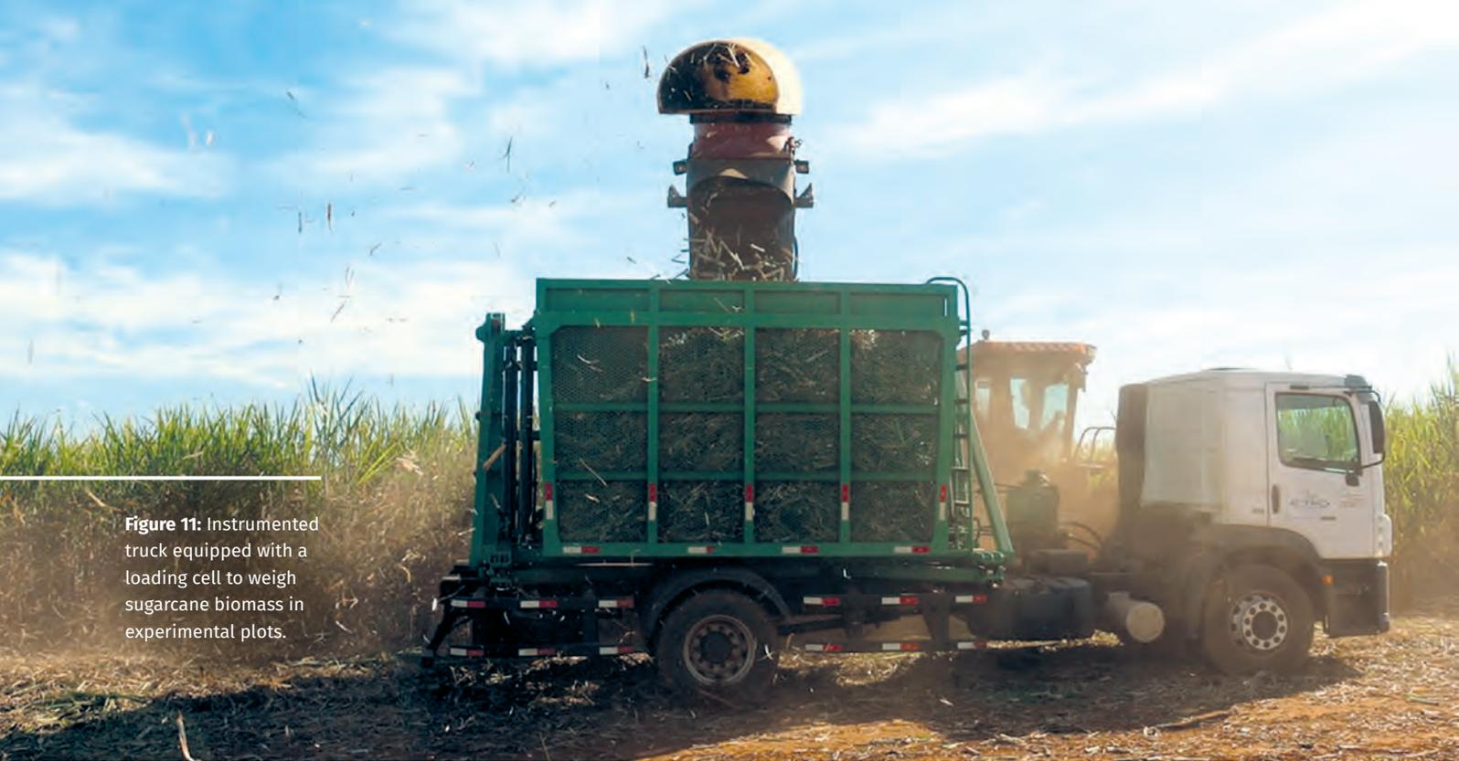
**Figure 11:** Instrumented truck equipped with a loading cell to weigh sugarcane biomass in experimental plots.
