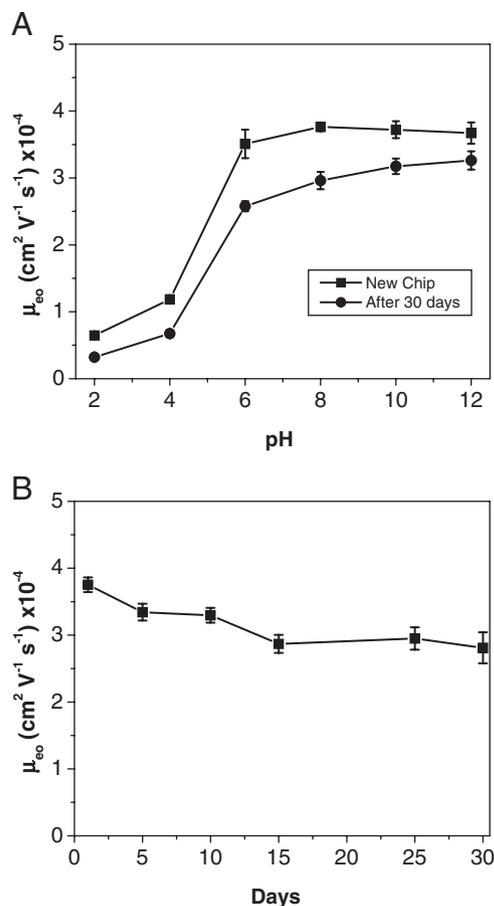
**Figure 6.** (A) Effect of the pH of the background electrolyte on the EOF magnitude measured by the current monitoring method for a new chip (■) and the same chip after 30 days (●). Each point in the graph is an average of six determinations; (B) EOF stability at pH 7 over the 30-day period.
