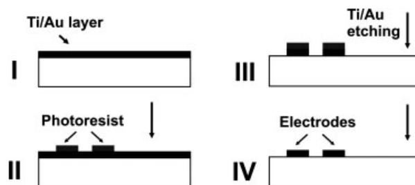
**Figure 3.** Fabrication process of gold electrodes on glass wafers. I, sputtering of a 20 nm titanium layer followed by 150 nm of gold; II, spin-coating of the PR layer; III, patterning of the PR step; IV, etch of the exposed Ti/Au followed by PR removing and washing steps.
