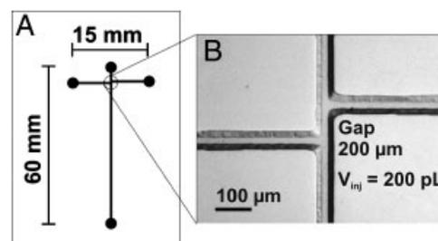
**Figure 1.** Presentation of the layout of the device (A), and its expanded view of the double-T injection system (B). The gap in the channel intersection was 200 μm.
