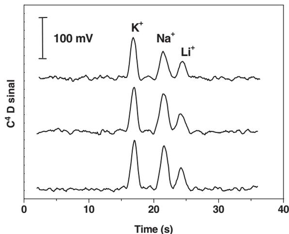
**Figure 8.** Electropherograms showing three consecutive separations of  $\text{Li}^+$ ,  $\text{Na}^+$  and  $\text{K}^+$  ( $100\ \mu\text{M}$  each) in a single chip using  $20\ \text{mM}$  MES/His as running buffer at pH 6.1. Injection:  $1\ \text{kV}/10\ \text{s}$  and separation at  $1\ \text{kV}$ . Detection was performed applying sinusoidal wave with frequency of  $120\ \text{kHz}$  and amplitude of  $2\ \text{V}_{\text{pp}}$ .
