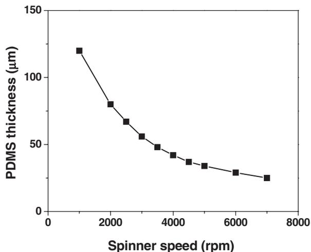
**Figure 5.** Thickness of the PDMS membrane in function of the spinner speed. The spinning time was 10 s.
