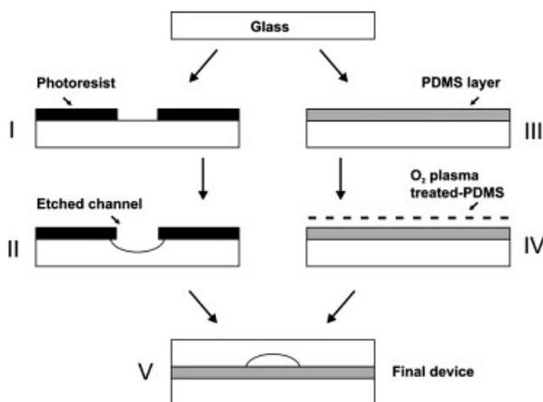
**Figure 2.** Microfabrication process of glass chip with sealing based on the use of a thin PDMS layer. I, patterning of PR step; II, wet chemical etching of glass with HF solution; III, spin-coating of a PDMS layer over flat glass surface at 3000 rpm during 10 s and baking at 100°C during 5 min; IV, plasma-oxidized PDMS during 1 min; V, final device after bonding step.
