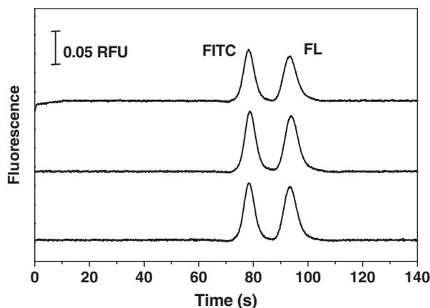
**Figure 7.** Electropherograms showing the repeatability on the separation of FL (50 μM) and FITC (150 μM) in a single chip. A 25 mM borate/boric acid was used as running buffer at pH 9. Injection and separation steps were performed by applying 1 kV/10 s and 2 kV, respectively. Detection was carried at 40 mm from the injection channel.
