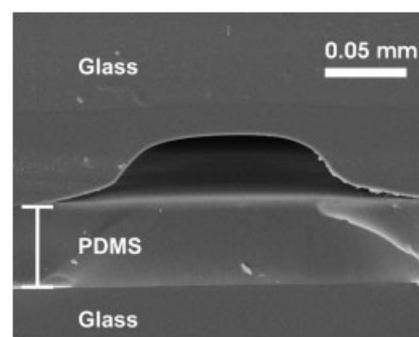
**Figure 4.** Scanning electron micrograph of the transversal section of the sealed glass channel with 135  $\mu\text{m}$ -wide at the opening of the channel, 85  $\mu\text{m}$ -wide at the bottom of the channel, and 35  $\mu\text{m}$ -deep the height of the channel.
