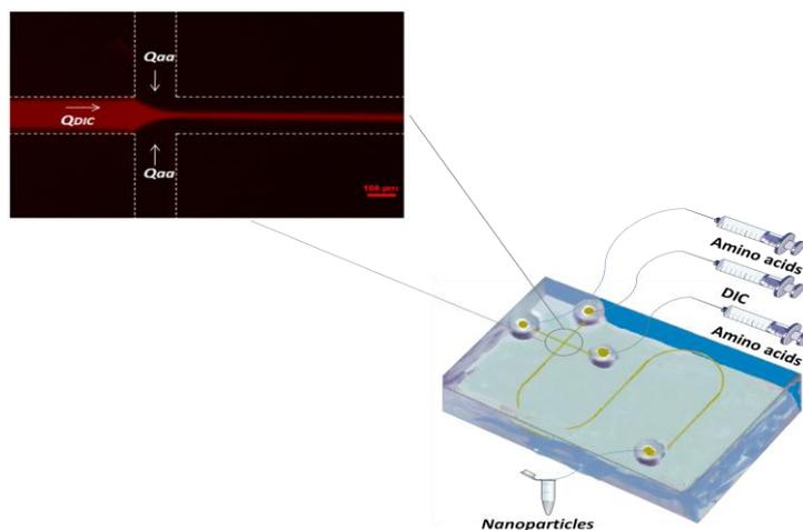
**Figure 1:** Synthesis of nanoparticles using microfluidic device based on hydrodynamic focusing.
