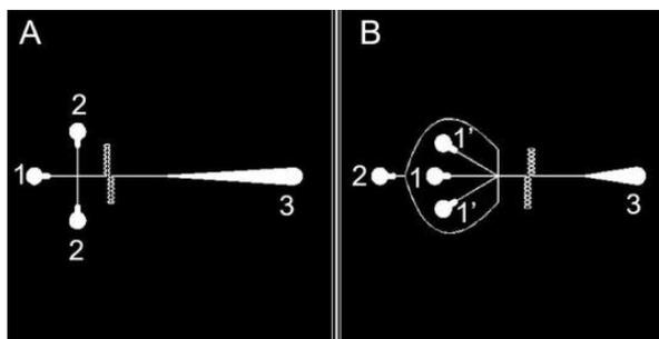
Figure 1. Design of the flow-focusing microchannels. A) Design 1 (inlet 1: aqueous phase (gellan solution); inlet 2: oily phase (soybean oil, PGPR and calcium acetate) and inlet 3: droplets collection chamber) and B) Design 2 (inlet 1: hydrophilic dye; inlet 1': gellan solution; inlet 2: oily phase (soybean oil, PGPR and calcium acetate) and inlet 3: droplets collection chamber).
