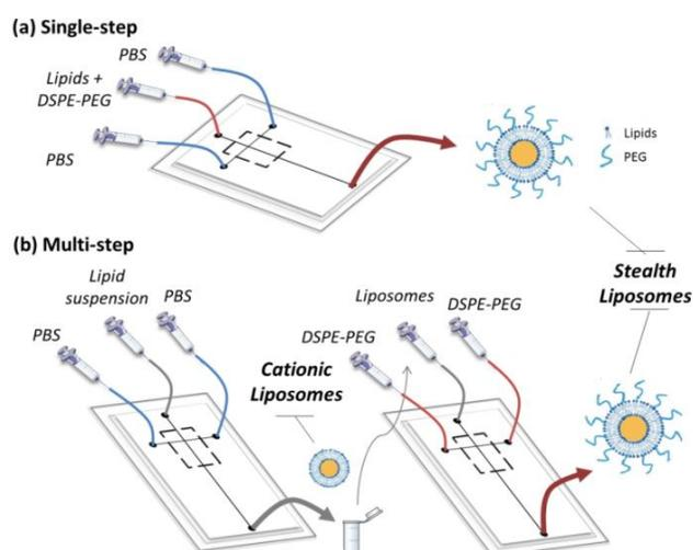
**Fig. 1.** Schematic diagram of single-step (a) and Multi-step (b) synthesis of stealth liposomes.
