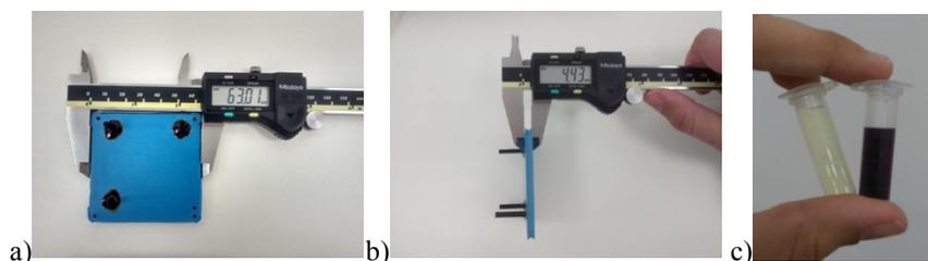
**Figure 1.** A,B) Microfluidic device fabricated with LTCC technology employed on synthesis of gold nanoparticles. C) Gold (III) salt used in nanoparticles synthesis and gold nanoparticles obtained through flow conditions.
