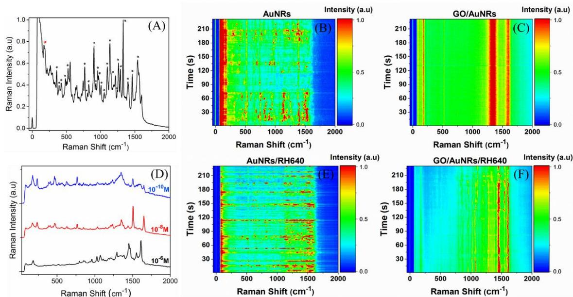
**Figure 1.** (a) SERS spectrum of the AuNR sample. The asterisks indicate the modes that are successfully assigned to CTAB. The red asterisk denotes the Au–Br stretching mode. SERS spectra time series for the (b) AuNR sample and (c) GO/AuNR nanocomposite sample. (d) Spectral comparison for different RH640 concentrations on the GO/AuNR nanocomposite. SERS spectra time series for (e) the AuNR/RH640 sample and (f) the GO/AuNR/RH640 sample
