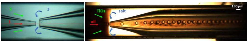
Figure 1: Emulsion production with microfluidic device.
