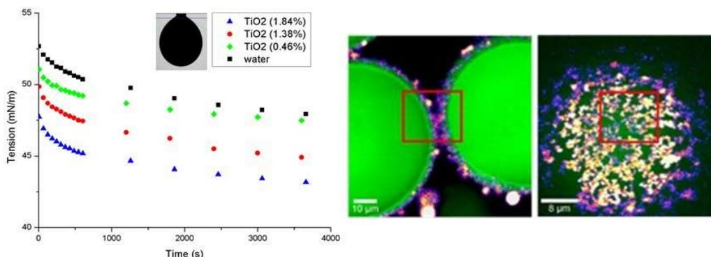
Figure 2: On the left: Interfacial tension of TiO<sub>2</sub> drop in oil, for different particle concentrations. On the right: Confocal Raman image of emulsion produced via traditional method: Oil droplet (in green) with TiO<sub>2</sub> “tentacles” (in purple) on the surface. The nanoparticles constitute a non-uniform coverage of the droplets surfaces of 2 to 4  $\mu\text{m}$  in thickness.
