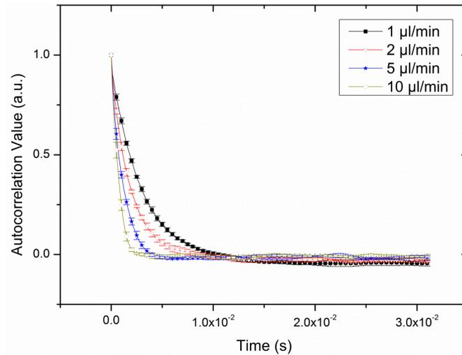
Fig. 2. Autocorrelation array for flows of 1  $\mu\text{l}/\text{min}$ , 2  $\mu\text{l}/\text{min}$ , 5  $\mu\text{l}/\text{min}$  and 10  $\mu\text{l}/\text{min}$ . Error bars are presented as  $\pm$  standard deviation.
