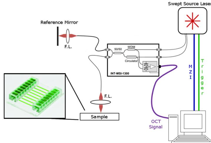
Fig. 1. OCT System setup illustration, with FL = Focusing Lens and WDM = Wavelength-division multiplexer. The inset shows the microfluidic device used in the tests.
