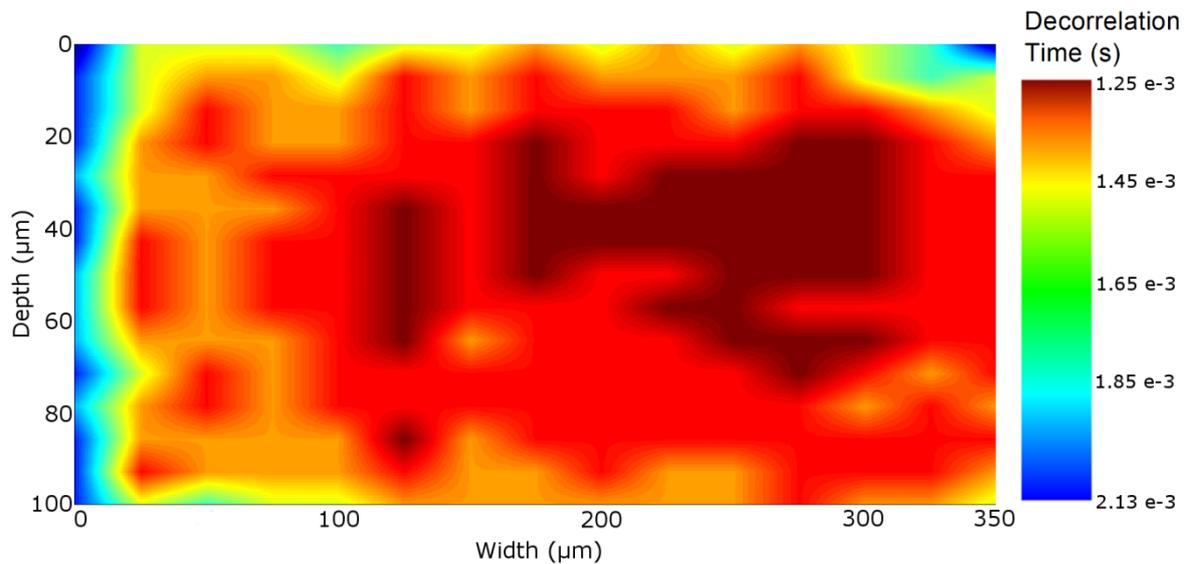
Fig. 4. Decorrelation time calculated for several points inside the microchannel while milk is pumped at 5  $\mu\text{l}/\text{min}$ . It functions as a B-Scan of flow gradient inside the microchannel.
