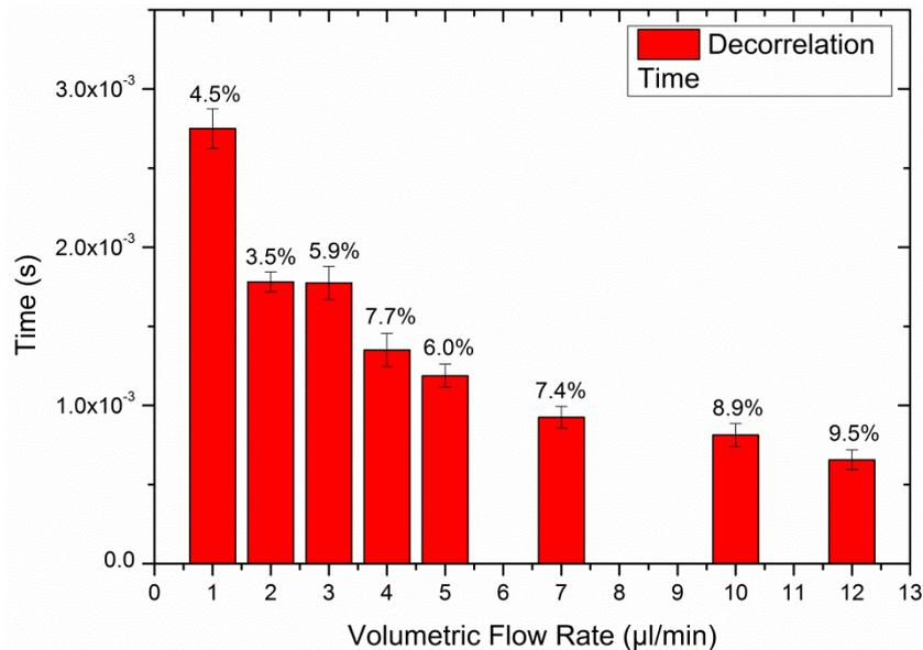
Fig. 3. Decorrelation time calculated for different flow rates. Note the trend of decrease with increasing volumetric flow. Error bars are presented as  $\pm$  standard deviation. Above each bar the Coefficient of Variation (in %) is reported.
