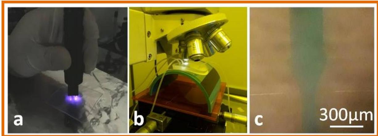
Fig 1. (a) PDMS surface treatment by atmospheric jet pressure plasma jet treatment; (b) Flexible device under optical microscopy inspection; (c) Microscopy image of the hydrodynamic focalization.
